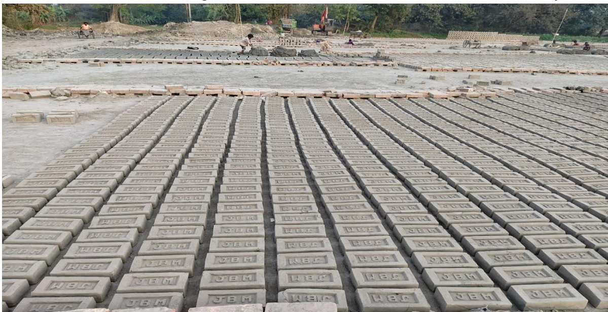
Moulded bricks waiting to be hard-burnt.
